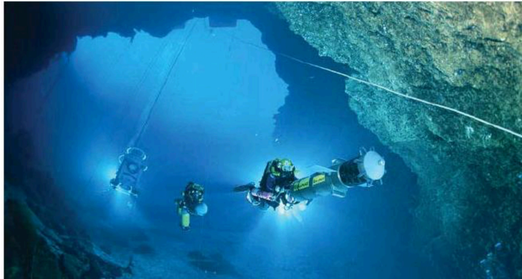
Heinerth guides the digital wall mapper, which produces 3D models of cave systems, at Wakulla Springs in Florida.
